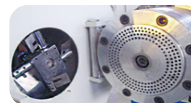
风冷切粒 Air-cooled cutting
