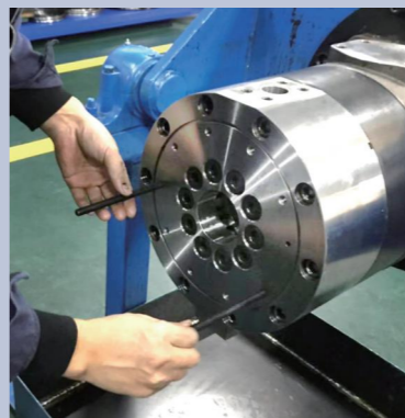
Reassemble HPS pump
