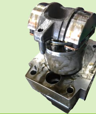
PV063 parker HPS pump dismantle
