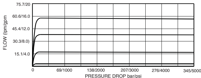
Flow Characteristics (Meter Out Mode) HEC12-32 with 5.5 Bar (80 psi) Spring 32cSt Oil at 40°C (104°F)
