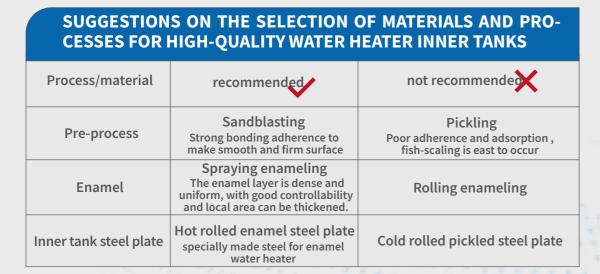
Gwippo suggests that the enterprise standard for glass-lined water heater is that the enamel should be customized designed as per production processes.
