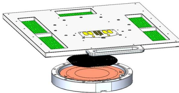
**Single-layer drawer design** Circuit of Each layer can be independently controlled, different single-layer works can be implemented in different modes, and different burn-in verification can be performed by scheduling the burn-in plan.
