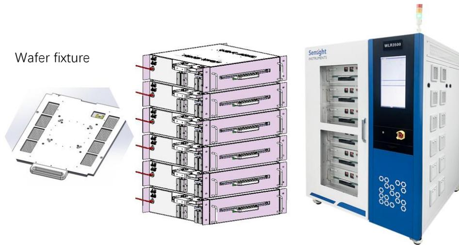
**Fixture design** The fixture is divided into two parts: the probe card and the heat sink, and the wafers can be combined via the Aligner equipment and placed in the burn-in system for burn-in.
