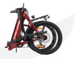
**Unfolding:** Unfold the main frame until the hinge joint is fully closed and lock it by pushing alloy lock lever until it clamps against the frame. Ensure the Saftey catch clicks into position and the lever cannot open.
