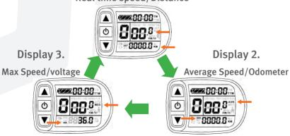
The Display will automatically switch back to display 1 after 5 seconds of inactivity.
