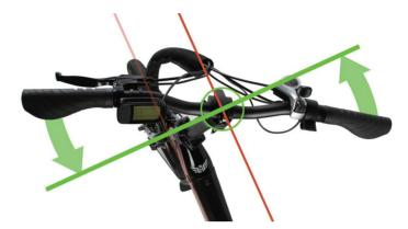
c. Once tight, unfold the handle bar again and secure with the QR lever against the stem post.d. Finally rotate the plastic safety lock ring until it engages and locks the alloy lock lever closed.
