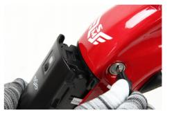
Before loading the battery, please make sure the key lock is in unlocked position. To secure the battery, please turn the key fully anticlockwise after loading the battery.
