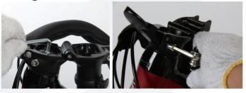
b. Carefully unfold the handlebar stem post up into its vertical position, Rotate the handlebars to sit perpendicular to the front wheel. Once satisfied the bars are correctly aligned, fold the bars down(without twisting) and retighten the stem screws.
